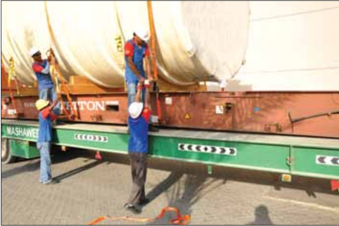
Specially trained CSS Group's lashing and crating team were assigned onsite for the lashing of over dimensional cargos like turbines, multi media filters, frontal piping skid, self cleaning filter skid, flocculation tanks which were more that 540 CBM loaded in trailers and also stuffed in 9 x 40 Ft high cube containers.
